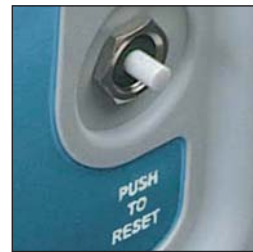
Circuit Breaker Reset
